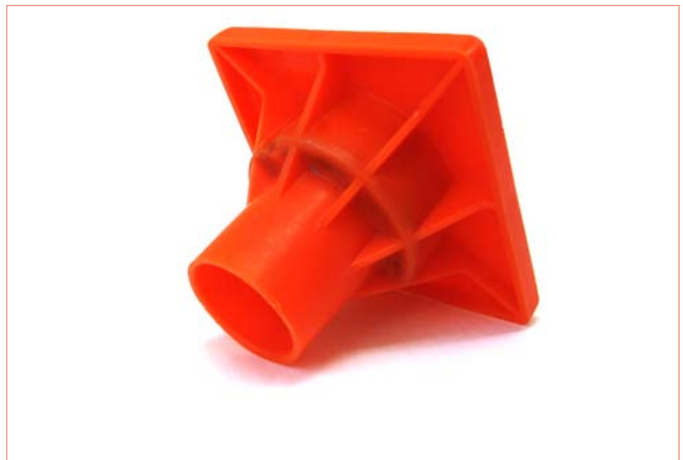
D-10 fits rebar #3-7, 3/8" to 7/8" diameter. *D-10 Protector Caps meets the testing requirements of CAL OSHA Construction safety orders section 1712 on impalement protection from concrete reinforcing bars (#3-9, 3/8" - 1 1/4") for heights up to 7 1/2" and 250 lbs. when properly installed.
